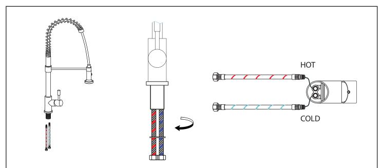
Insert Hot & Cold Hoses into Faucet and Tighten. Follow placement on Hot and Cold Hose as per the diagram.
